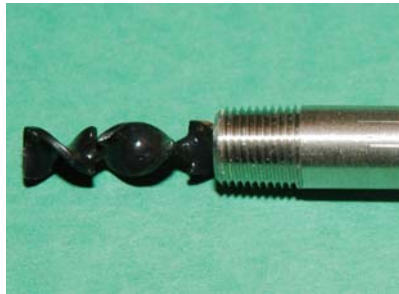
Figure #15: Type HT Helical Static Mixer In metal construction in pipe with MNPT End Connections. . Right Photo – Teflon® coated 316 S/S mixing element to minimize fouling with materials that cling to metal surfaces.
