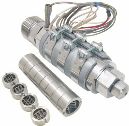
Figure #1: StaMixCo Injection Molding Mixing Nozzle with eight (8) Mixing Elements, Heater Bands and Thermocouple.
