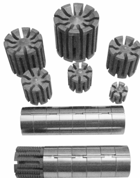
Figure #4: SMF Filter-SMN Mixing Element combination used to retain particles to protect hot runner system and tools when processing regrind material.
